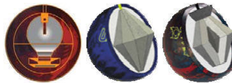
Figure 2: Example core shapes that will be modeled by calculating rotational moments of inertia. 8,9
