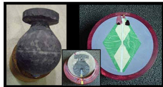
Figure 4: Example ball cores that will or have been extracted and will be tested on the rotational dynamics platform. Theoretical calculations based on the 3-dimensional core shape will also be conducted and compared to the experimental results.
